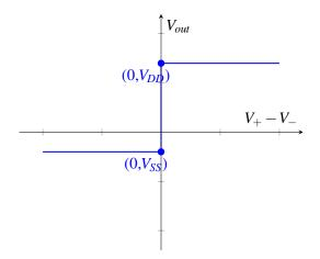
For any ideal op-amp, when  $V_+ < V_-$  ( $V_+ - V_- < 0$ ), we have  $V_{out}$  equals  $V_{SS}$ ; when  $V_+ - V_- > 0$ , we have  $V_{out}$  equals  $V_{DD}$ . If we zoom in around  $V_+ - V_- = 0$  by a million times, we will be able to see there is actually some finite slope associated with the transition region.
