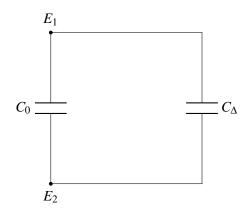
If we consider the parallel combination of  $C_0$  and  $C_{\Delta}$  as some equivalent capacitance  $C_{eq}$ , we know that  $C_{eq}$  will have some value greater than  $C_0$  because  $C_{eq} = C_0 + C_{\Delta}$  and  $C_{\Delta} > 0$ .
