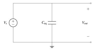
We can immediately see that no matter how  $C_{eq}$  changes, the voltage measured  $V_{out}$  is always going to be equal to  $V_s$ .
