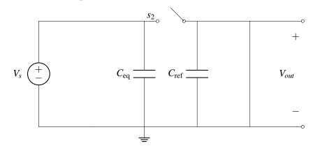
In this phase, the voltage across  $C_{eq}$  is  $V_s$ , and the voltage across  $C_{ref}$  is zero.
