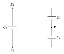
Since we care about the circuit behavior at nodes  $E_1$  and  $E_2$ , we can further simplify the circuit by replacing the series combination of  $C_1$  and  $C_2$  with some capacitance  $C_{\Delta} = \frac{C_1 C_2}{C_1 + C_2}$ .
