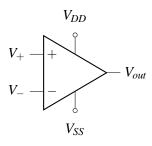
We have two input terminals named  $V_+$  and  $V_-$ , two power supply terminals named  $V_{DD}$  and  $V_{SS}$ , and one output terminal named  $V_{out}$ . The op-amp circuit can transform a voltage signal  $(V_+ - V_-)$  into  $V_{out}$ . For the op-amp to function correctly, we need to connect the two external voltage sources  $V_{DD}$ ,  $V_{SS}$  to the op-amp (typically  $V_{DD} > 0$  and  $V_{SS} \le 0$ ). The symbol actually represents the following equivalent circuit:
