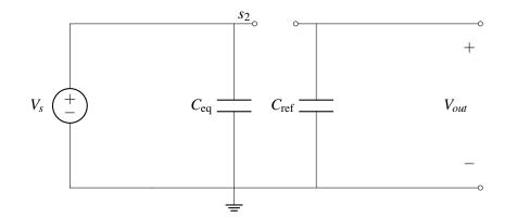
In phase 1,  $C_{eq}$  is connected to voltage source  $V_s$  and  $C_{ref}$  is not connected to anything. – **Phase 2:**  $s_1$  is open and  $s_2$  is closed.
