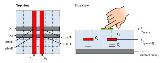
Given 4 pixels and their corresponding locations, we can measure the capacitance at  $(x_1, y_1)$  to know if there is a finger pressing on top of pixel 1. Similarly, to know if there is a finger pressing on top of pixels 2, 3, 4, we can measure the capacitances at  $(x_1, y_2)$ ,  $(x_2, y_1)$ ,  $(x_2, y_2)$ . If we sense an increase in the capacitance at the pixel location, we know there is a finger pressing on top of this pixel.
