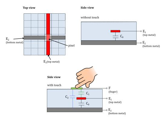
Our finger touches the dielectric at the top,  $C_2$  is the capacitance between our finger (*F*) and electrode  $E_2$ , and  $C_1$  is the capacitance between our finger (*F*) and electrode  $E_1$ . Now, we can draw the equivalent circuit model corresponding to the pixel we're looking at:
