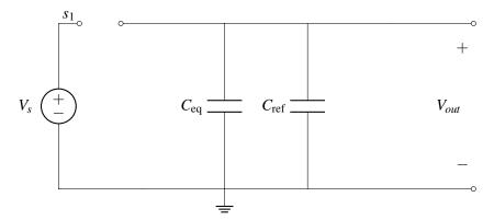
In phase 2,  $C_{eq}$  is disconnected from  $V_s$  and  $C_{ref}$  is connected to  $C_{eq}$ . However, there is one serious problem with this circuit, since we are not sure what is the initial charge of  $C_{ref}$ , we cannot perform any circuit analysis. Our second attempt fails because the initial condition of  $C_{ref}$  is not clear.
