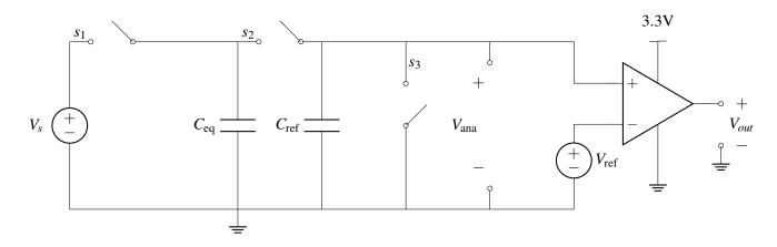
Since the two input voltages to the op-amp are the output of the circuit  $V_{ana}$ , and our threshold voltage  $V_{ref}$ , if the voltage  $V_{ana}$  is greater than  $V_{ref}$ , the output voltage  $V_{out}$  will be 3.3 V. If  $V_{ana} < V_{ref}$ ,  $V_{out}$  will be 0V. Recall for  $V_{ana}$ , we have
