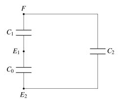
A smart phone can only sense something that is between electrodes  $E_1$  and  $E_2$  as it is impractical to physically connect a measuring device to our finger. So, we redraw our circuit as follows:
