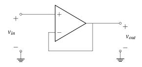
To analyze this circuit, we first notice that  $u_+ = v_{in}$  and  $u_- = v_{out}$ . We apply the second golden rule,  $u_+ = u_-$ , which tells us
