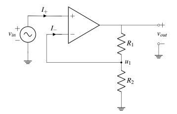
For the non-inverting amplifier circuit, we have
