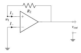
**Step 2: "Dink"**  $v_{out}$ . If we increase  $v_{out}$ , we know  $u_1$  is going to increase because  $u_1 = v_{out}$ .  $u_1$  is connected to  $u_+$ , so  $u_+$  increases, therefore  $v_{in} = u_+ - u_-$  increases, and thus  $v_{out}$  increases. So the feedback from the circuit is in the same direction, this circuit is in positive feedback.
