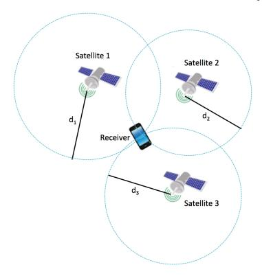
However, in real life, our measurements will be noisy. Can we use extra measurements from more satellites to reduce the effects of noise? In this module, we'll also look at how to combine many measurements together to get a better estimate of position.
