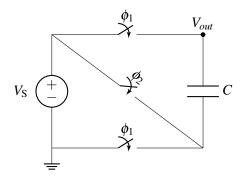
(a) In the circuit above switches  $\phi_1$  are initially closed and switch  $\phi_2$  is initially open. Calculate the value of the output voltage,  $V_{out}$  with respect to ground, and the amount of charge stored on capacitor, *C*, at that state (phase 1).
