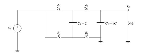
In the first phase, all of the switches labeled  $\phi_1$  will be closed and all switches labeled  $\phi_2$  will be open. In the second phase, all switches labeled  $\phi_1$  are opened and all switches labeled  $\phi_2$  are closed.
