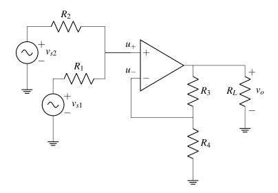
(a) First, let's focus on the left part of the circuit containing the voltage sources  $v_{s1}$  and  $v_{s2}$ , and resistances  $R_1$  and  $R_2$ . Solve for  $u_+$  in the circuit above. (*Hint: Use superposition.*)
