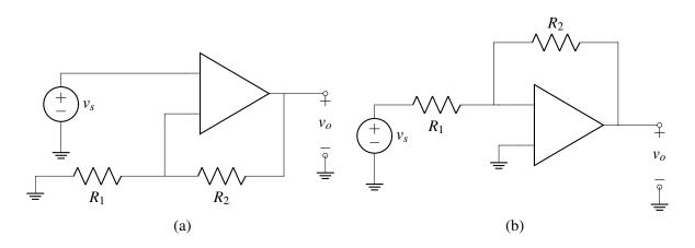
(a) Label the input terminals of the op-amp with (+) and (-) signs in Figure (a), so that it is in negative feedback. Then derive the voltage gain  $(G = \frac{v_o}{v_s})$  of the non-inverting amplifier in Figure (a) using the Golden Rules. Why do you think this circuit is called a non-inverting amplifier?
