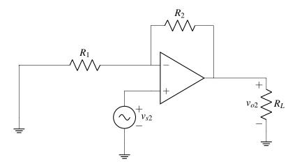
(c) Use the Golden Rules to find the output voltage  $v_o$  for the circuit shown below.
