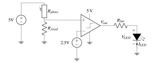
Note  $R_{photo}$  is a photoresistor, which acts like a typical resistor but changes resistance based on the amount of light it is exposed to. This photoresistor is located inside the kitchen drawer, so we can tell when the drawer is opened or closed.
