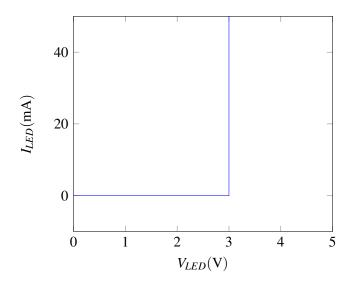
To avoid exceeding the power rating of the LED (and having it burn out), the recommended value for  $I_{LED}$  is 20 mA.
