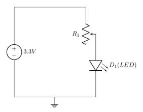
This circuit is known as an **LED Fader Circuit**. This circuit has three nodes and three circuit elements (a voltage source, a resistor and an LED). The arrow on top of the resistor means that this is a **variable resistor**; *i.e.*, it does not have a fixed value. Let's look at a couple of the circuit elements you will be using in this lab:
