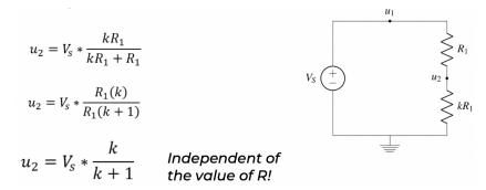
Thus, we can see that the voltage between two resistors whose resistances are multiples of each other is independent of the actual resistances. It only depends on the scaling factor k.
