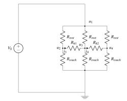
All we need to do now is to measure the voltages at different points in this circuit to determine what point is being touched. However, we are not quite done with building our touchscreen. We saw earlier that the voltages differ in the vertical direction but not in the horizontal direction. This means that we can only find unique points in the vertical direction. How do we uniquely determine pairs of points along both axes? What if we flip the orientation of the touchscreen by  $90^{\circ}$ ?
