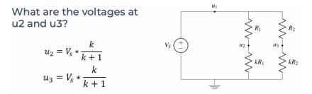
Please refer to Note 14 if you are confused about these derivations. Now, say we connected another resistor  $R_3$  between nodes  $u_2$  and  $u_3$ . What would the current be through that resistor? Think about the potential difference across that resistor; *i.e.*,  $V_{u_2} - V_{u_3}$ .
