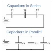
For series,  $\frac{1}{C_{eq}} = \frac{1}{C_1} + \frac{1}{C_2} + ... + \frac{1}{C_n}$
