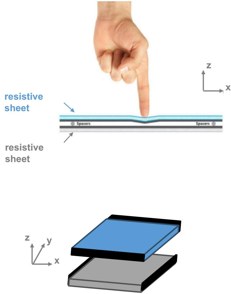
Our circuit model for each resistive sheet is a grid of resistors:
