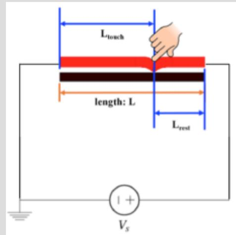
Model 2 - imperfect conductor (resistor)
