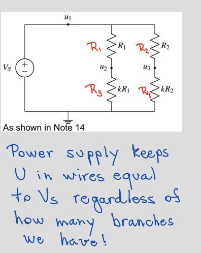
$$U_{2} = \frac{R_{3}}{R_{1} + R_{3}} \cdot V_{5}$$
