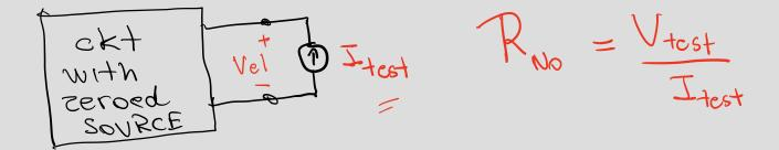
Circuit Analysis Method – What happens when we have multiple Voltage or Current sources?
