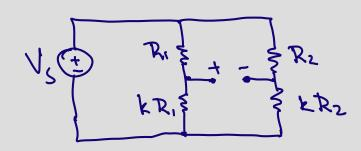
Elems = resistor (Rs) Vels = U2-U3 (Voltage Des.) Bold Assumption  $V_{e}V_{5} = 0$ if Vels = 0 = Jels = Vels = 0 Rs if Jols = 0 The circuit is the same as the one we already analysed without Rs. We showed :  $U_2 = U_3$  $Vels = V_2 - V_3 = O$
