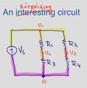
. What are U2 and U3 ?  $U_2 = R_3$ . Us  $R_1 + R_3$ V3 = Ru. Vs R2+Ry  $V_{2}-O = \frac{R_{3}}{R_{3}} \cdot (V_{1}-O)$ RitR3  $U_3 - O = \frac{R_4}{R_2 + R_4} \cdot (U_1 - O)$  $V_1 - 0 = V_S$
