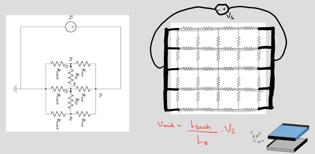
Connecting voltage source to top sheet gives *y*-*touch* position Connecting voltage source to bottom sheet gives *x*-*touch* position
