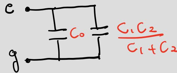
Equivalent capacitance for C<sub>1</sub> in series with C<sub>2</sub>
