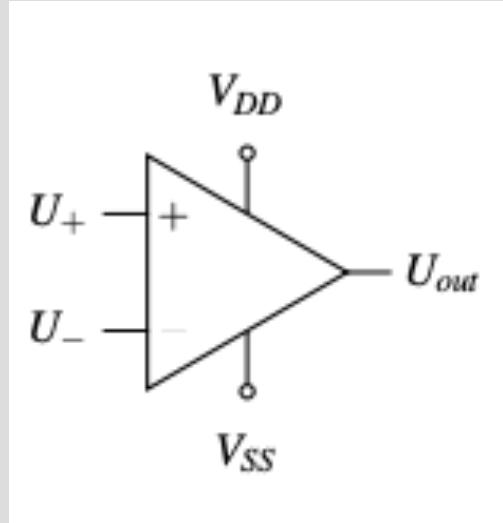
An op-amp has two input terminals marked (+) and (-) with potentials  $U_+$  and  $U_-$ , two power supply terminals called  $V_{DD}$  and  $V_{SS}$ , and one output terminal with potential  $U_{out}$ .
