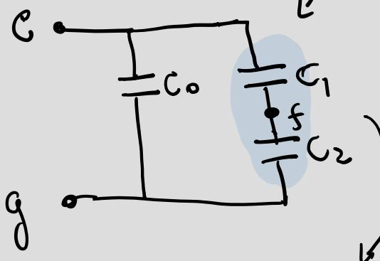
Redraw to focus on terminals (nodes) e and g
