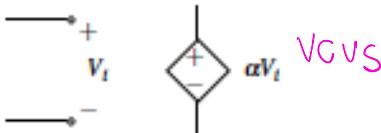
Voltage-controlled voltage source
