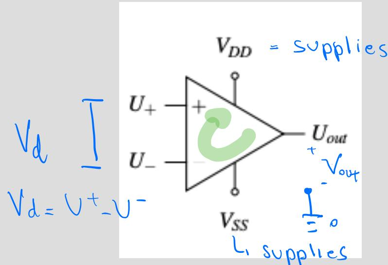
An op-amp has two input terminals marked (+) and (-) with potentials  $U_+$  and  $U_-$ , two power supply terminals called  $V_{DD}$  and  $V_{SS}$ , and one output terminal with potential  $U_{out}$ .
