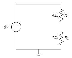
3. In the same circuit as above, how much power is dissipated in the voltage source?
