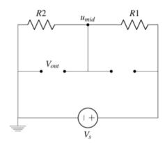
Does the voltage at  $u_{mid}$  change in this case? Thinking about it in terms of nodal analysis, we have not actually added any new nodes to our circuit - ideal wires (with zero voltage drop) are all that we have actually added. Therefore, we see that with a perfect conductor (analogous to our ideal wire),  $V_{out} = u_{mid}$ . Note here that  $V_{out}$  is the voltage drop across an open circuit that is placed in parallel with resistor  $R_2$  to capture  $V_{R_2} = u_{mid}$ .
