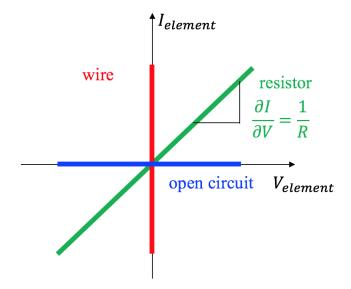
From the I-V plots, although a resistor, a wire and an open circuit can behave quite differently, their behaviors are exactly the same at (0, 0). This means that at (0, 0), these three circuit elements can be replaced by one another and the same behavior (I = 0, V = 0) is still expected.
