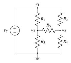
• Step 2: Write equations for the nodes with voltage sources between them. Here, the ground node and  $u_1$  have  $V_s$  between them, which tells us that
