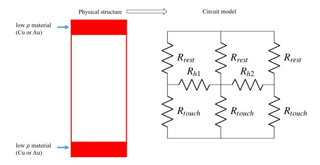
As we did with the 1D touchscreen, we connect a voltage supply  $V_s$  to the top and bottom ends of the top red plate:
