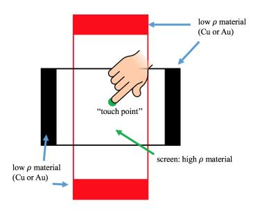
The top and bottom ends of the top red plate as well as the left and right ends of the bottom black plate are made of materials that have very low resistivities  $\rho$ , we can treat them as ideal wires ( $\rho = 0$ ). The materials of the transparent screen that we touch in the middle have much higher resistivity.
