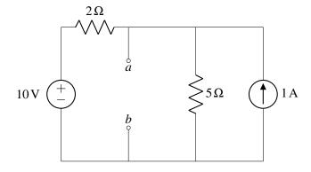
8. For the same circuit above, what is the equivalent Thevenin resistance between the nodes a and b?
