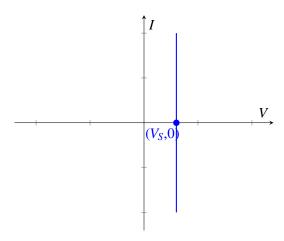
Now if we want to zero out this voltage source, we are setting  $V_S = 0$ . Then the I-V plot is exactly the y-axis.
