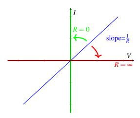
We know that the slope of the line is equal to  $\frac{1}{R}$ . What happens in the limit where R trends towards infinity? Then the line becomes the x-axis, which corresponds to an open circuit as we've seen earlier. Now what happens in the limit where R trends towards zero? The line becomes the y-axis, which corresponds to a wire.
