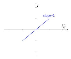
An important implication of this is that current is only flowing through the capacitor if the voltage across the capacitor is changing with time. If the voltage is no longer changing, then the current through the capacitor will equal 0.
