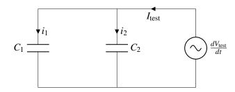
$$i_1 = C_1 \frac{dV_{test}}{dt}$$
