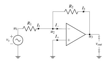
For the inverting amplifier circuit, we have
