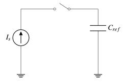
When the switch closes at t = 0, we start charging the capacitor. The voltage over the capacitor will indicate how much time has elapsed since the switch closed (i.e. since the button was pressed).
