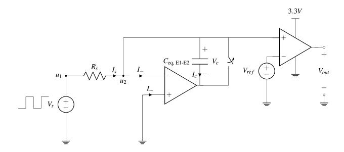
Let's look at the comparator/op-amp on the right side. Note that its positive terminal is directly connected to  $u_2$ , and  $u_2 = 0$  V. This means that  $u_+$  of the right-most comparator op-amp is always zero and does not depend on the capacitance  $C_{\text{eq,E1-E2}}$ . Therefore,  $V_{out}$  cannot detect changes in  $C_{\text{eq,E1-E2}}$  and the circuit does not work as intended.
