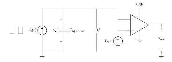
Here the current source,  $I_s$ , outputs a periodic square wave alternating between  $I_1$  and  $-I_1$  every T/2 seconds. The voltage over the capacitor  $V_c$  increases linearly, with a slope that depends on  $C_{\rm eq, E1-E2}$ . The switch is opened at  $t=\frac{T}{4}$ .
