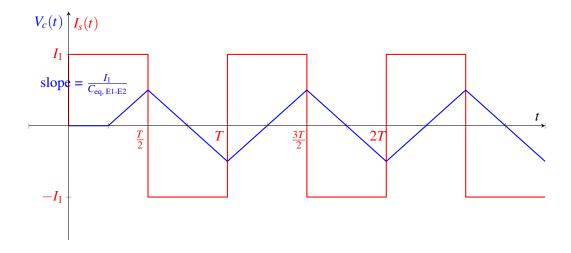
The periodic current source is critical in this design, but not readily available. Can we use our design of the "almost" current source in our capacitive touchscreen? The "almost" current source outputs a constant current, while we need a periodic current (shown in red above). However, we can achieve this by powering the "almost" current source with a periodic voltage instead of a constant voltage:
