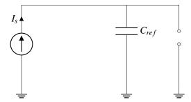
This change in circuit architecture has another important benefit: it guarantees that the initial voltage on the capacitor is 0 V. We used this assumption when setting  $V_{ref}$  in Eq.(3). Without this change, we would not know the initial voltage, and therefore we could not choose  $V_{ref}$  to correctly correspond to 2 sec.
