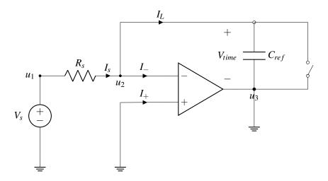
Let's consider the case after the button is pressed and the switch is open. We are supposed to be charging the capacitor to keep track of time. However,  $u_3$  is connected to ground, and  $u_2 = 0$  V by the second golden rule. Therefore, the voltage across  $C_{ref}$  is
