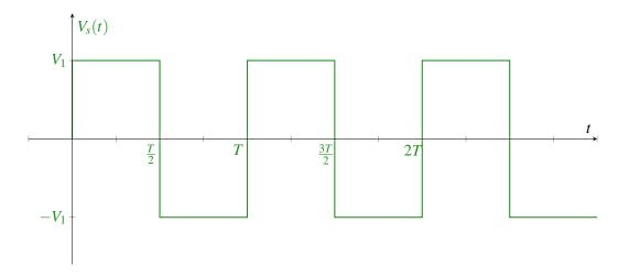
Since  $I_s = \frac{V_s}{R_s}$ , the current supplied to the load element will be either  $\frac{V_1}{R_s}$  or  $-\frac{V_1}{R_s}$ . Now let's attach this current source to our touchscreen circuit.
