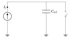
Before the button is pressed, the switch is closed and can be replaced by a wire. In this case, the current from the current source can flow through this wire to ground, eliminating the prior contradiction. In addition, when the switch is closed, it connects the top of the capacitor to ground, so the voltage across the capacitor remains constant at  $0\,\mathrm{V}$ .
