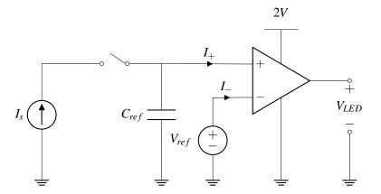
We choose  $V_{ref}$  to be set equal to the voltage on the capacitor after charging for 2s (assuming the capacitor is initially uncharged):
