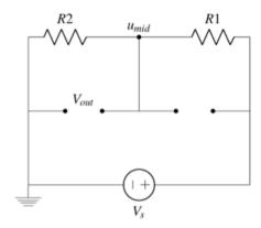
So why have the bottom plate at all? It lets us take the measurement for  $V_{out}$  using connection points on the edge of the plate instead of having to put a probe or wire at the actual touch point every time! As we have shown, in the case of an ideal bottom plate this does not affect the measurement result itself.
