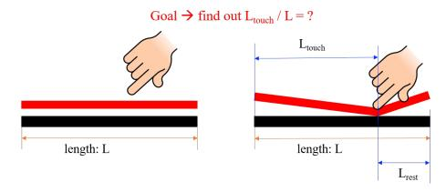
Previously, we ignored the black "bottom plate"; But why do we want it at all? Let's return to the model of our touchscreen and build from that. The simple version is shown below, where  $u_{mid}$  represents the point where the finger is touching. Note that a voltage source has been connected around it, with the positive terminal connected to one edge of the top plate and the negative terminal connected to the opposite edge.
