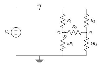
Once again, we could analyze this circuit from scratch using our circuit analysis procedure, but maybe we can simplify the analysis. Let's make a bold assumption that adding  $R_3$  will not affect circuit operation and therefore  $u_2 = u_3$  from our analysis above. We can determine if this assumption is true by analyzing the circuit and seeing if there are any contradictions that arise. If there are no contradictions, then we know that this bold assumption is true.
