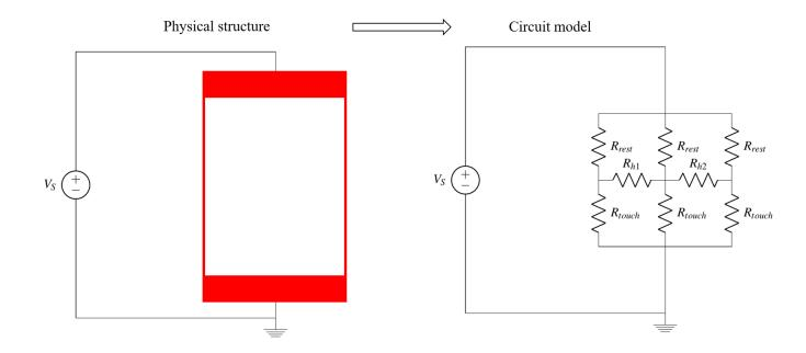
Let's analyze the circuit we just built with the top red plate and a voltage supply  $V_s$ :
