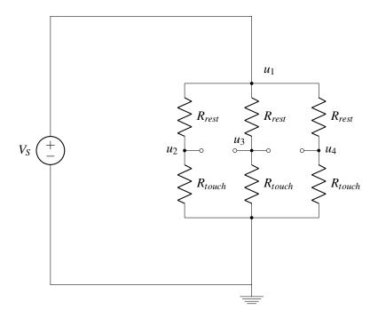
After replacing horizontal resistors with open circuit, we can use a voltmeter and measure  $u_3$ . Once again, using the voltage divider equation, we get:
