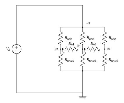
Does this circuit remind you of the "interesting circuit" we analyzed in the previous section? Since  $R_{rest}$  and  $R_{touch}$  are the same for each segment, we know that  $u_2 = u_3 = u_4$ . As with the "interesting circuit" can replace horizontal resistors  $R_{h1}$ ,  $R_{h2}$  with open circuits.
