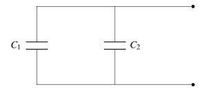
What is the equivalent capacitance? By analogy with our resistor case, we will try and apply a test voltage to this circuit:
