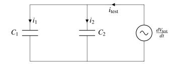
$$i_1 = C_1 \frac{dV_{test}}{dt}$$
