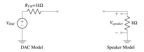
In this example, we'd like  $V_{speaker} = V_{DAC}$ , so that the DAC output is directly played on the speaker. We try connecting the DAC and speaker together directly:
