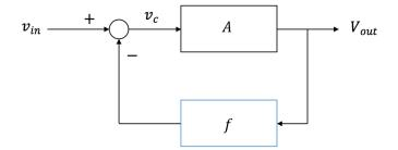
We have negative feedback gain f. For an op-amp in negative feedback, we have
