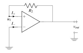
**Step 2** "dink  $v_{out}$ " If we increase  $v_{out}$ , we know  $u_1$  is going to increase because  $u_1 = v_{out}$ .  $u_1$  is connected to  $u_+$ , so  $u_+$  increases, therefore  $v_{in} = u_+ - u_-$  increases, and thus  $v_{out}$  increases. So the feedback from the circuit is in the same direction, this circuit is in positive feedback.
