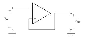
To analyze this circuit, we first notice that  $u_+ = v_{in}$  and  $u_- = v_{out}$ . We apply the second golden rule,  $u_+ = u_-$ , which tells us
