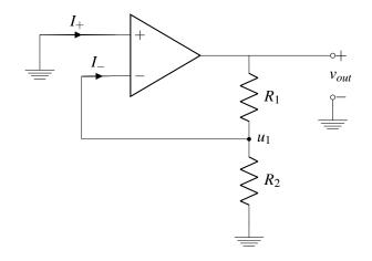
**Step 2** "dink  $v_{out}$ " If we increase  $v_{out}$ , we know  $u_1$  is going to increase because  $R_1$  and  $R_2$  form a voltage divider circuit.  $u_1$  is connected to  $u_-$ , so  $u_-$  increases, therefore  $v_{in} = u_+ - u_-$  decreases, and thus  $v_{out}$  decreases. So the feedback from the circuit is in the opposite direction, this circuit is in negative feedback.
