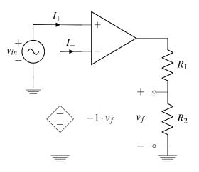
**Step 1** Zero out all **independent** sources. We cannot zero out controlled voltage source  $-1 \cdot v_f$  because this is not an independent voltage source.
