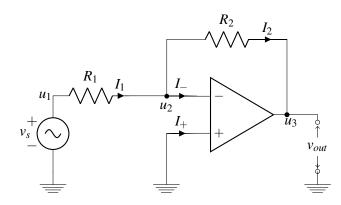
Let's assume that this circuit is in negative feedback so that we can use golden rule #2, after analyzing the circuit we will show how to check if a circuit is indeed in negative feedback. We know that by applying KCL, we have
