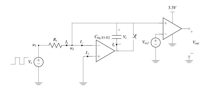
Let's look at the op-amp on the right side. Note that it's positive terminal is directly connected to  $u_2$ , and  $u_2 = 0$ . This means that  $u_+$  of the right most op-amp is always zero and does not depend on the capacitance  $C_{\text{eq,E1-E2}}$ . Therefore,  $V_{out}$  cannot detect changes in  $C_{\text{eq,E1-E2}}$  and the circuit does not work as intended.
