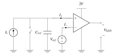
Can you build this countdown timer in lab? Almost! The only thing that is missing is the current source. In the next section, we'll explore building an ideal current source out of commonly available components.
