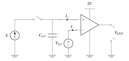
We choose  $V_{ref}$  to be set equal to the voltage on the capacitor after charging for 2s (assuming the capacitor is initially uncharged):
