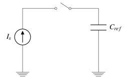
When the switch closes at t = 0, we start charging the capacitor. The voltage over the capacitor will indicate how much time has elapsed since the switch closed (i.e. since the button was pressed).
