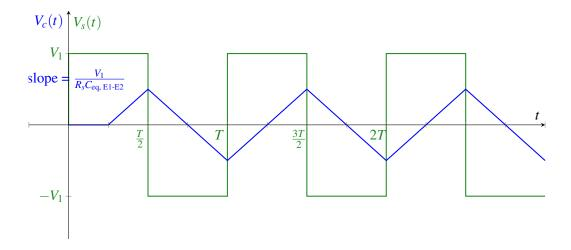
Recalling that  $C_{\text{eq, E1-E2}}$  increases when there is a touch, we can plot  $u_+ = -V_c$  when the finger is present and absent. We'd like to set  $V_{ref}$  halfway between the peak of  $u_+$  with a touch and  $u_+$  without a touch.
