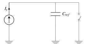
Before the button is pressed, the switch is closed and can be replaced by a wire. In this case, the current from the current source can flow through this wire to ground, eliminating the contradiction that happened before. In addition, when the switch is closed, it connects the top of the capacitor to ground, so the voltage drop over the capacitor remains constant at 0.
