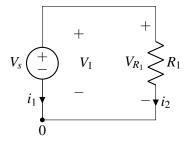
(c) Suppose we choose a second labeling of the circuit as shown below. Calculate the power dissipated or supplied by every element in the circuit. Let  $V_s = 5 \text{ V}$  and let  $R_1 = 5 \Omega$ .
