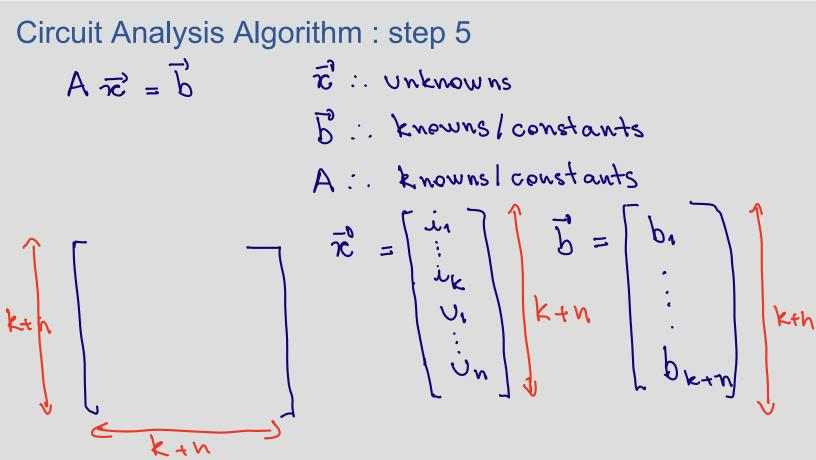
Use KCL to fill as many rows of A as possible (linear independence) # Nodes -1 = N-1
