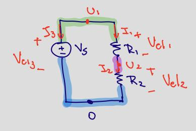
\* Importan Passive sign convention: the current enters at the positive terminal and exits are the negative terminal.
