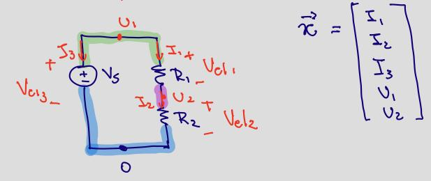
Passive sign convention: the current enters at the positive terminal and exits are the negative terminal.
