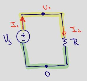
Add signs + and – element voltages to each element following the passive sign convention
