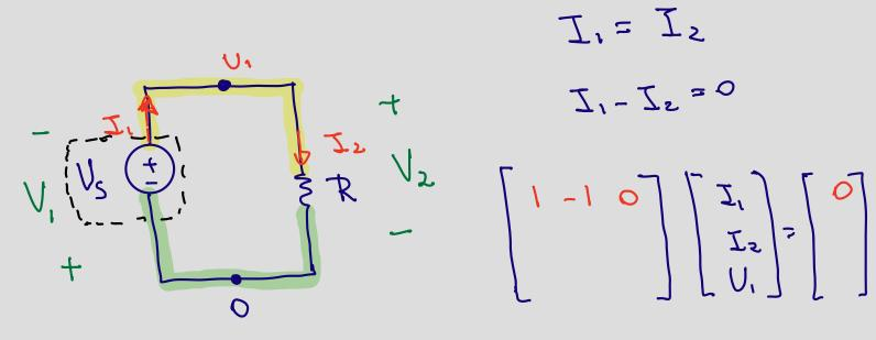
Use current-voltage relationships for each element to fill the rest of the A matrix
