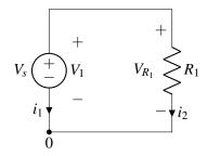
(c) Suppose we choose a second labeling of the circuit as shown below. Calculate the power dissipated or supplied by every element in the circuit. Again, let  $V_s = 5 \,\mathrm{V}$  and let  $R_1 = 5 \,\Omega$ .
