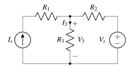
(a) With the current source turned on and the voltage source turned off, find the current  $I_3$ .
