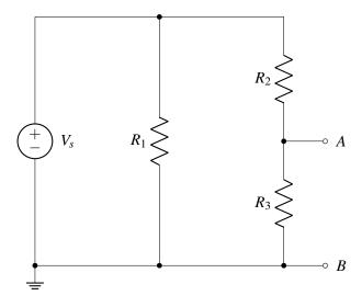
(b) Now a load resistor,  $R_L$ , is connected across terminals A and B, as shown in the circuit below. Using Thévenin equivalence, find the power dissipated in the load resistor in terms of the given variables.
