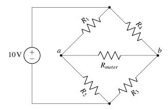
Unfortunately, you voltmeter is far from ideal, so  $R_{meter} = 4k\Omega$ . Is the voltage  $V_{ab}$  you found in part (a) equal to the new voltage  $V_{R_{meter}}$  across the voltmeter resistor? Why or why not? Calculate the current  $I_{R_{meter}}$  through the voltmeter resistor and the voltage  $V_{R_{meter}}$  across the meter resistor.
