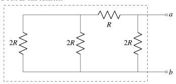
(c) Find the equivalent resistance looking in from points a and b. In other words, express the resistive network in the dashed box as one resistor.
