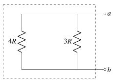
(b) Find the equivalent resistance looking in from points a and b. In other words, express the resistive network in the dashed box as one resistor.
