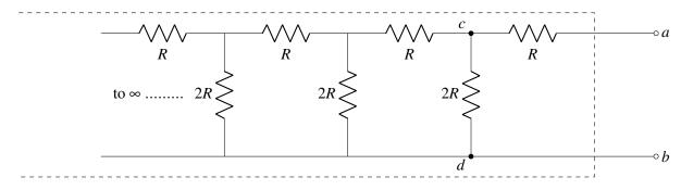
As a first step you can replace the circuit looking to the left from c and d by  $R_{in1}$ .
