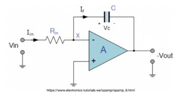
Let's go over the circuit equations for this circuit to see why we can use it for our touchscreen. Using golden rule #1, we see that both  $V^+ = 0V$  and  $V^- = 0V$ . Applying KCL on the  $V^-$  node:
