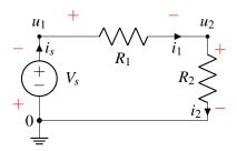
**Definition 11.4 (Passive Sign Convention):** The **passive sign convention** dictates that positive current should *enter* the positive voltage terminal and *exit* the negative voltage terminal of an element. Below is an example for a resistor:
