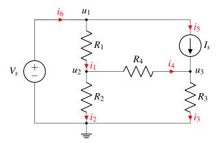
**Step 4:** Label element potentials based on passive sign convention.
