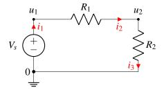
Note that we only label the current once for each element—for example, we can label  $i_3$  as the current leaving the resistor (as is done in the diagram) or we can label it as the the current entering the resistor. These are equivalent because KCL also holds within the element itself—i.e., the current entering an element must be equal to the current exiting that same element.
