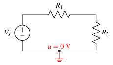
**Step 2:** Label all remaining nodes as some " $u_i$ ", representing the voltage at each node relative to the zero/reference node.
