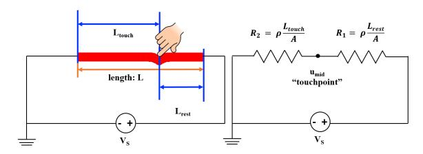
By using a voltage divider circuit, we can map  $u_{mid}$  to  $L_{touch}$ . A relationship between  $u_{mid}$  and  $L_{touch}$  exists such that:
