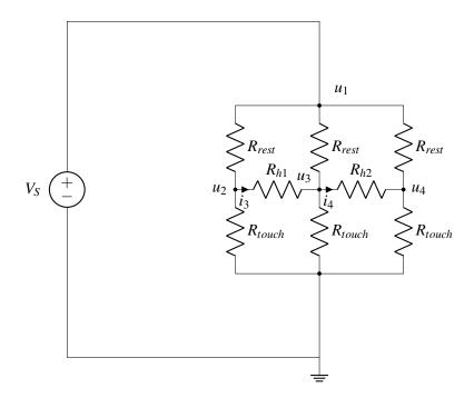
Does this circuit remind you of the "interesting circuit" we analyzed in the previous section? Since  $R_{rest}$  and  $R_{touch}$  are the same for each segment, we know that  $u_2 = u_3 = u_4$ . As with the "interesting circuit" can replace horizontal resistors  $R_{h1}$ ,  $R_{h2}$  with open circuits.
