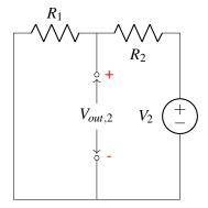
We again recognize that this is just a voltage divider circuit and therefore we can see that  $V_{out,2} = \frac{R_1}{R_1 + R_2} V_2$ . Finally, to get the output voltage  $V_{out}$  of the original circuit, we add the contributions from each voltage source  $V_{out} = V_{out,1} + V_{out,2} = \frac{R_2}{R_1 + R_2} V_1 + \frac{R_1}{R_1 + R_2} V_2$ .
