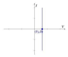
Now if we want to zero out this voltage source, we are setting  $V_S = 0$ . Then the I-V plot is exactly the y-axis.
