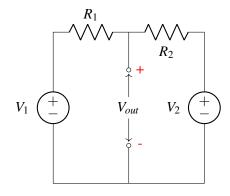
We first compute the output voltage due to  $V_1$  and hence source  $V_2$  will be replaced with a wire:
