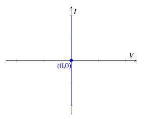
What does this mean? This means that it allows any current to go through, however the voltage drop always remains zero. This is exactly what a wire element (sometimes called a short circuit) does.
