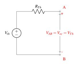
**Step 2, find**  $R_{Th}$ : Zero out any independent sources. Remember, this means voltage sources turn into a wire and current sources turn into an open circuit. Then apply either a test current into the terminal and measure the resultant voltage, or apply a test voltage and measure the resultant current.  $R_{Th} = \frac{V_{test}}{I_{tot}}$
