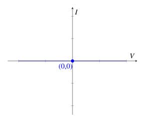
What does this mean? This means no matter what voltage you apply, there will be no current. This is equivalent to an open circuit.
