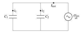
$$i_1 = C_1 \frac{dV_{test}}{dt}$$
