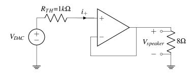
From the first golden rule, we know that  $i_+ = 0$ . This means there is no current through  $R_{TH}$ , and therefore no voltage drop across the resistor. In other words, the op-amp does not load the DAC since it has infinite internal resistance (remember that we model the input terminals as floating nodes)! Since there is no voltage drop over  $R_{TH}$ , we know that  $u_+ = V_{DAC}$ . Combing this with our previous analysis of the buffer, we see that  $V_{DAC} = V_{speaker}$ , as desired.
