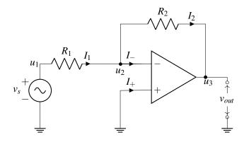
For the inverting amplifier circuit, we have
