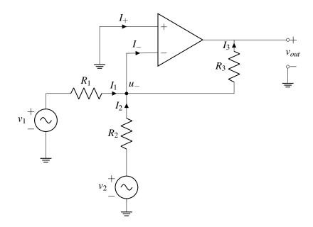
Let's analyze this circuit. First, let's apply the first golden rule,  $I_{-} = I_{+} = 0$ . Applying KCL at the node labelled  $u_{-}$ , we have
