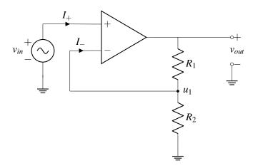
For the non-inverting amplifier circuit, we have
