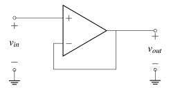
To analyze this circuit, we first notice that  $u_+ = v_{in}$  and  $u_- = v_{out}$ . We apply the second golden rule,  $u_+ = u_-$ , which tells us
