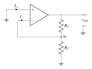
**Step 2: "Dink"**  $v_{out}$ . If we increase  $v_{out}$ , we know  $u_1$  is going to increase because  $R_1$  and  $R_2$  form a voltage divider circuit.  $u_1$  is connected to  $u_-$ , so  $u_-$  increases, therefore  $v_{in} = u_+ - u_-$  decreases, and thus  $v_{out}$  decreases. So the feedback from the circuit is in the opposite direction, this circuit is in negative feedback.
