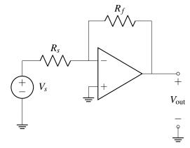
2. In the circuit above, if  $R_s = 50 \Omega$ ,  $R_f = 100 \Omega$ , and  $V_s = 2 V$ , what is the value of  $V_{out}$ ?
