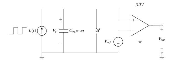
Here the current source,  $I_s$ , outputs a periodic square wave alternating between  $I_1$  and  $-I_1$  every T/2 seconds. The voltage over the capacitor  $V_c$  increases linearly, with a slope that depends on  $C_{\text{eq, E1-E2}}$ . The switch is opened at  $t = \frac{T}{4}$ .
