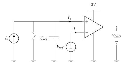
Can you build this countdown timer in lab? Almost! The only thing that is missing is the current source. In the next section, we'll explore building an ideal current source out of commonly available components.
