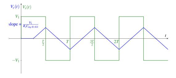
Recalling capacitance  $C_{\text{eq, E1-E2}}$  increases when there is a touch, we can plot  $u_+ = -V_c$  when the finger is either present or absent. We'd like to set  $V_{ref}$  halfway between the peak of  $u_+$  with a touch and  $u_+$  without a touch.
