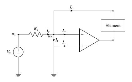
In this case,  $I_L$  will become 0 A because all of the current will flow through the wire between  $U_-$  and  $U_+$  (in other words,  $I_1 = I_s$ ). Therefore we cannot physically connect  $U_-$  to ground.
