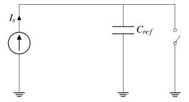
Before the button is pressed, the switch is closed and can be replaced by a wire. In this case, the current from the current source can flow through this wire to ground, eliminating the prior contradiction. In addition, when the switch is closed, it connects the top of the capacitor to ground, so the voltage across the capacitor remains constant at 0 V.
