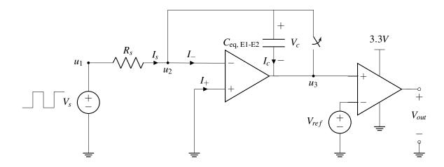
By the second golden rule (applied to the left op-amp),  $u_2 = U_+ = 0$  V. We can use KVL to determine that
