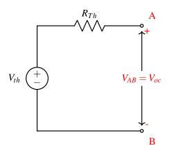
**Step 2, find**  $R_{Th}$ : Zero out any independent sources. Remember, this means voltage sources turn into a wire and current sources turn into an open circuit. Then apply either a test current into the terminal and measure the resultant voltage, or apply a test voltage and measure the resultant current.  $R_{Th} = \frac{V_{test}}{I_{test}}$
