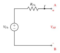
Now how would you figure out  $V_{Th}$  and  $R_{Th}$  for the Thevenin equivalent circuit?
