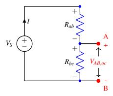
Note that the same current flows through the two resistors. In addition, the voltage drop over the two resistors sums to  $V_s$ , so we can write  $V_{Rab} = V_s - V_{AB,oc}$ . Therefore, using Ohm's Law:
