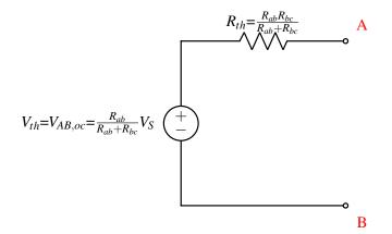
This is not the same result! In this case, the Thevenin voltages in the two circuits are different. This example shows how different pairs of nodes in the same circuit result in different equivalent circuits. In general, there is no guarantee that circuits will behave in the same way from the standpoint of different pairs of nodes.
