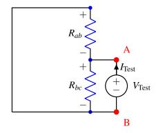
We can see that this is the same as the parallel resistor case we examined above: therefore,  $R_{Th} = \frac{V_{\text{Test}}}{I_{\text{Test}}} = R_{ab} \parallel R_{bc}$ .
