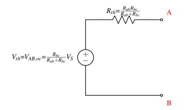
What if we instead chose the upper two nodes (instead of the lower two nodes) as the two terminals (nodes A and B)? We can follow the same procedure to find an equivalent Thevenin circuit from the standpoint of these new nodes,
