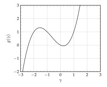
The  $g(\cdot)$  is the only nonlinearity in this system. We want to linearize this entire system around a operating point/equilibrium. Any point  $\vec{x}_{\star}$  is an operating point if  $\vec{f}(\vec{x}_{\star}(t), u_{\star}(t)) = \vec{0}$ .
