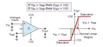
You will use a comparator to compare the output of the DAC to the analog input voltage you get from the potentiometer.
