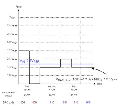
Figure 5: Timing diagram of SAR output code. The red digit in the DAC code is the bit being decided in the current conversion cycle; blue digits are the bits determined by the previous conversion cycles.
