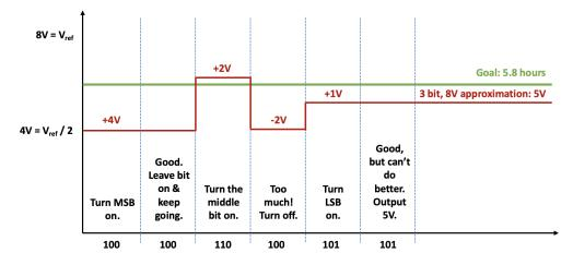
Figure 6: DAC output as SAR ADC algorithm progresses for an input of 5.8V
