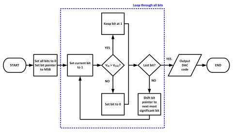
Figure 3: Flow chart of SAR ADC algorithm
