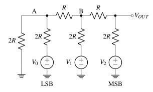
Figure 1: 3-bit DAC built from R-2R ladder
