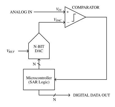
Figure 2: SAR ADC circuit diagram
