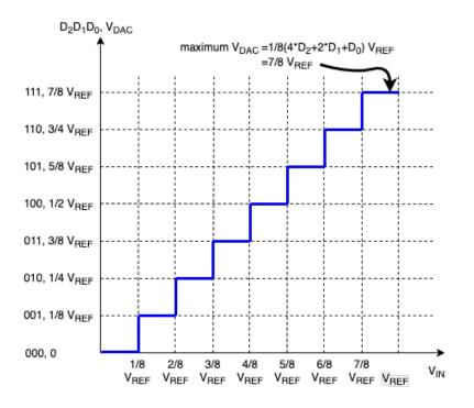
Figure 4: Voltage transfer curve of 3-bit SAR ADC
