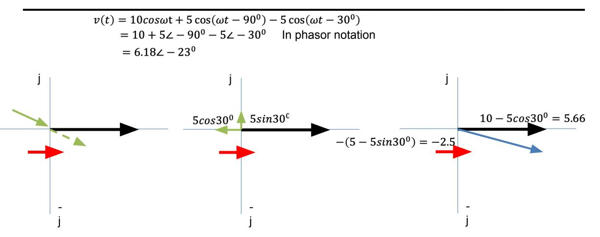
Phasors are like vectors where the phase angle denotes the angle between coordinate axes with j representing  $90^{\circ}$
