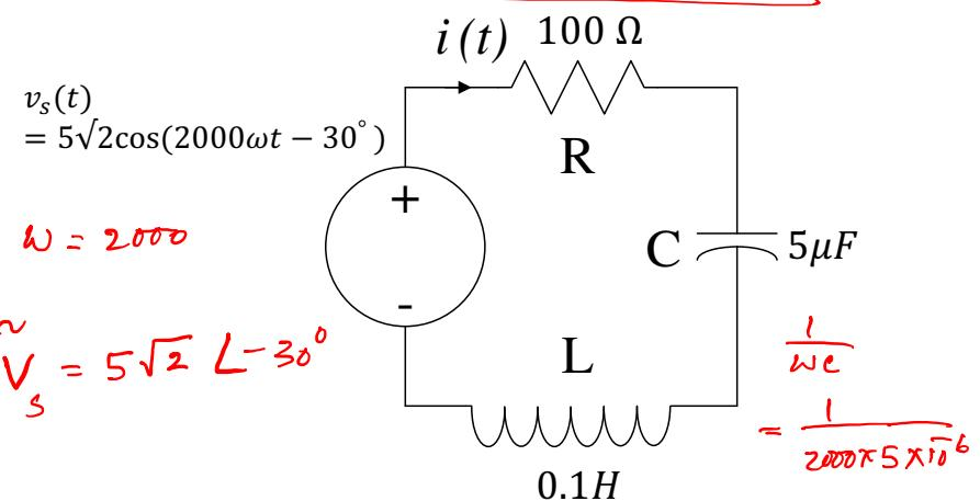
$$\begin{aligned} \omega L &= 2000 \times 0.1 &= \frac{1}{1/\omega_0} \\ &= 200 &= 100 \end{aligned}$$
