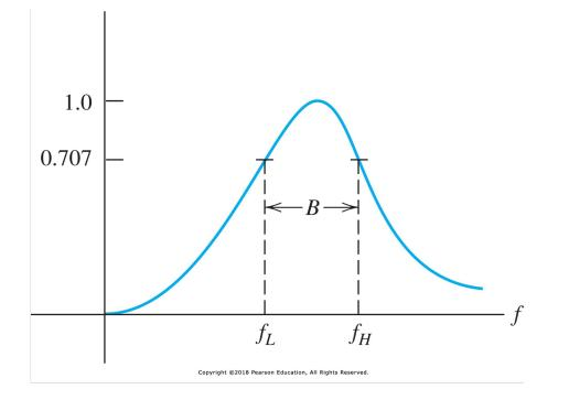
**Half-power** frequencies are defined as the frequencies where the magnitude of the transfer function has fallen by a factor of  $\frac{1}{\sqrt{2}} = 0.707$
