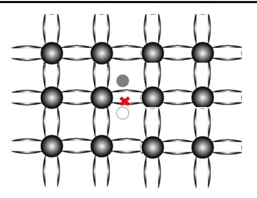
At finite temperature, an electron may gain enough energy to break the covalent bond, become free and move around.
