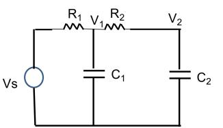
$$V_1 = I_2 R_2 + V_2 = R_2 C_2 \frac{dV_2}{dt} + V_2$$
