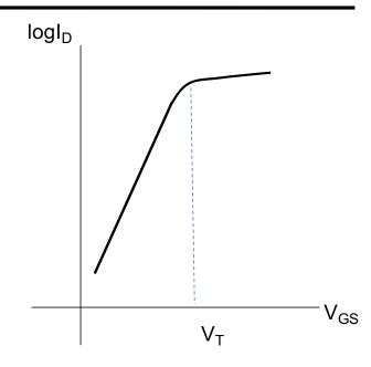
When  $V_{GS}$  is High,  $R_{SD}$  is low When  $V_{GS}$  is Low,  $R_{SD}$  is High
