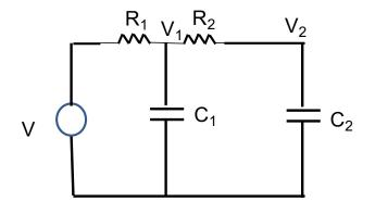
$$\frac{dV_1}{dt} = -\left(\frac{1}{R_2C_1} + \frac{1}{R_1C_1}\right)V_1 + \frac{1}{R_2C_1}V_2 + \frac{1}{R_1C_1}V_S$$
