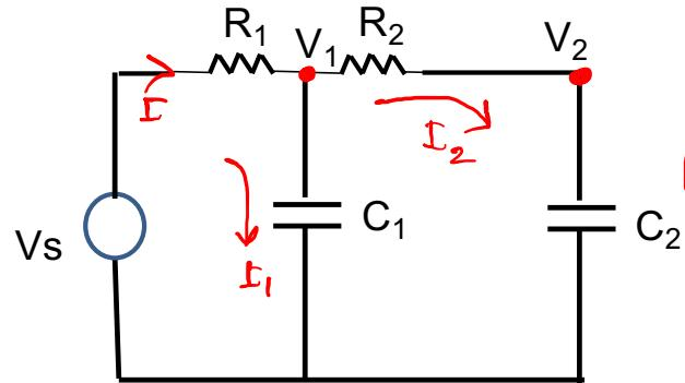
$$V_1 = I_2 R_2 + V_2 = R_2 C_2 \frac{dV_2}{dt} + V_2$$
