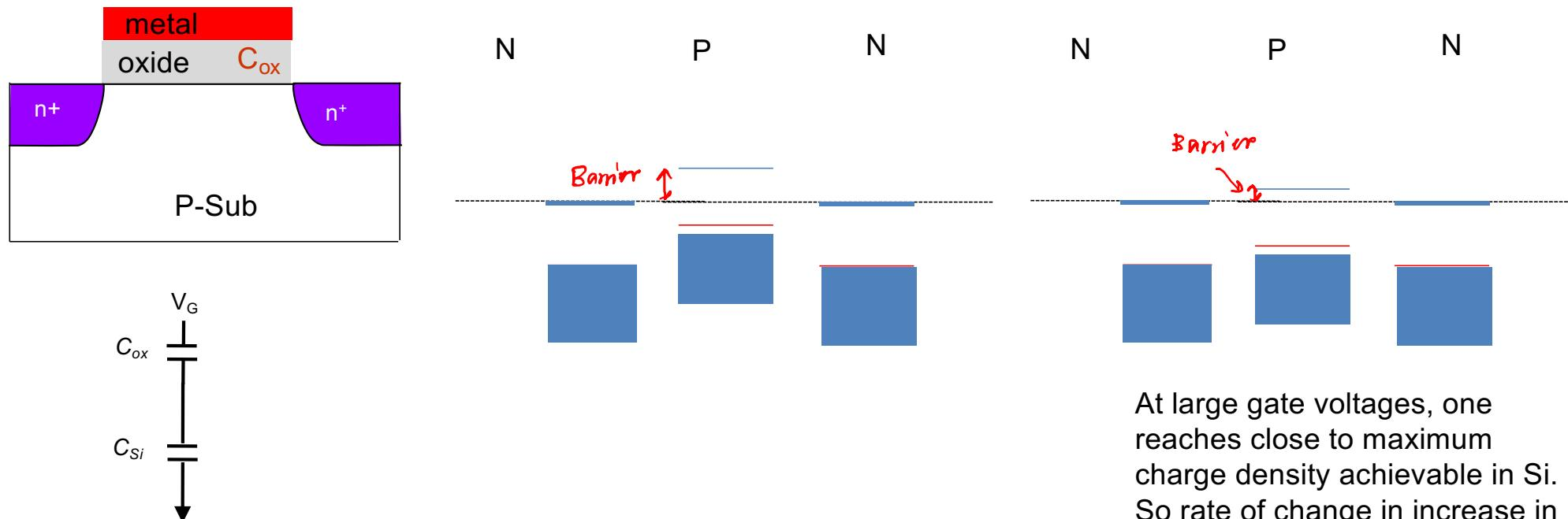
At large gate voltages, one reaches close to maximum charge density achievable in Si. So rate of change in increase in electron density with gate voltage slows down
