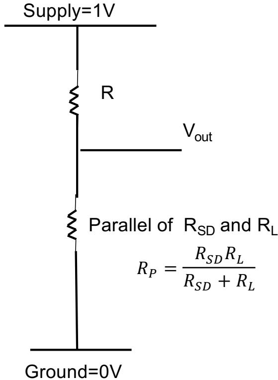
$$V_{out} = \frac{R_P}{R + R_P} V_{supply}$$
