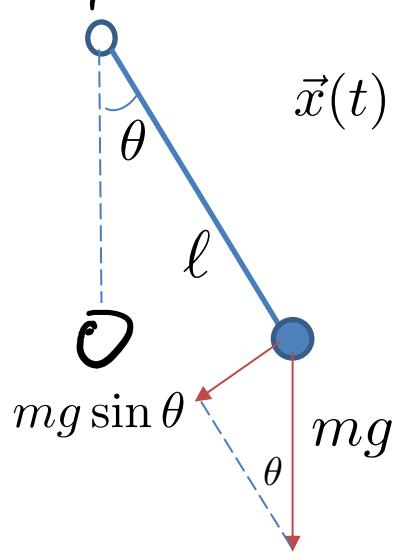
$$\vec{x}(t) = \begin{bmatrix} x_1(t) \\ x_2(t) \end{bmatrix} = \begin{bmatrix} \theta(t) \\ \frac{d\theta(t)}{dt} \end{bmatrix} \in \mathbb{R}^2 \quad \left\{ \begin{array}{l} \frac{dx_1(t)}{dt} = x_2(t) \\ \frac{dx_2(t)}{dt} = -\frac{g}{l} \sin(x_1(t)) - \frac{k}{m} x_2(t) \end{array} \right. \quad \begin{array}{l} = f_1(x_1(t), x_2(t)) \\ = \underline{f_2(x_1(t), x_2(t))} \end{array}$$
