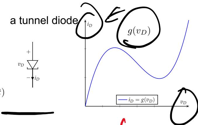
$$\left\{ \begin{array}{l} \frac{dx_1(t)}{dt} = \frac{1}{C} (x_2 - g(x_1)) \\ \frac{dx_2(t)}{dt} = \frac{1}{L} (u - R x_2 - x_1) \end{array} \right. \quad \begin{array}{l} (=0) \\ (=0) \end{array}$$
